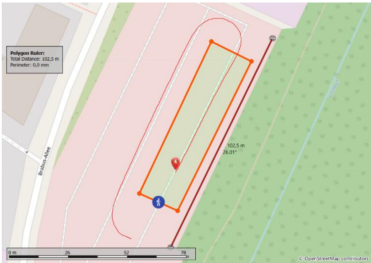
Figure 3-1: Test route displayed in OpenStreetMap, showing the position of the pedestrian, the position of the vehicle, the vehicle's trajectory (red line), and the test area (orange rectangle). All measurements were conducted within the test area. The total length of the test track is approximately 100 metres, with the measuring area spanning about 70 metres.
