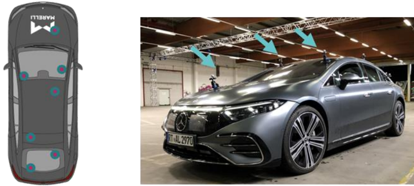
Figure 3-14: Test vehicle with IR reflectors. Schematic positions (left), vehicle inside test venue with reflectors attached (right).
