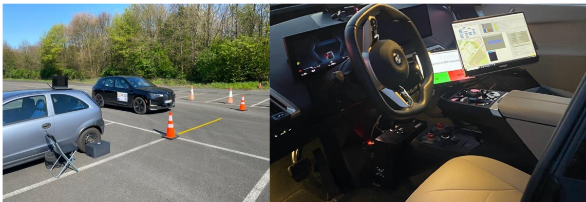
Figure 3-3: Test setup in the area of the pedestrian crossing and the interior of the test vehicle with the TFT for visualising the questions on distraction to the driver as well as the control screen for the test supervisor.
