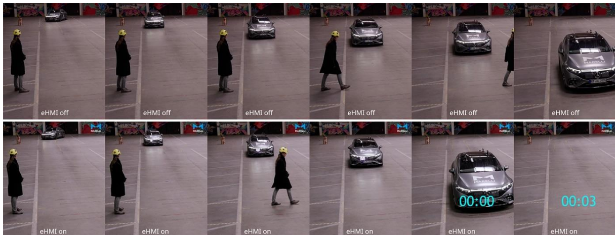
Figure 3-24: Side by side comparison between Interactions w/ and w/o eHMI active. On resolution of the situation w/ eHMI the timer starts. W/o eHMI the situation takes three seconds longer to resolve.
