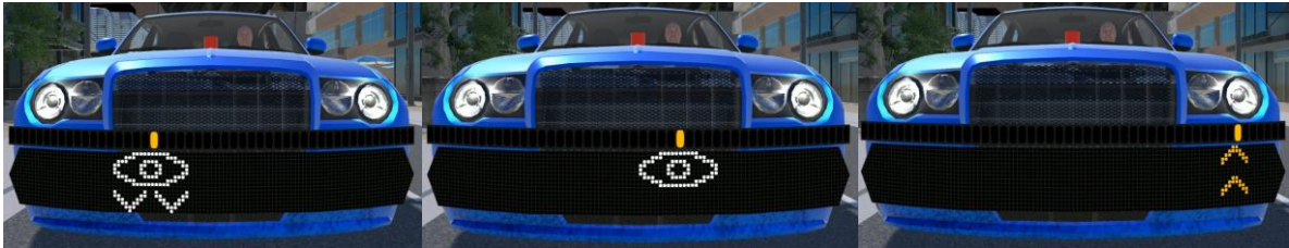
Figure 3-17: HMI 2 – Long-Term eHMI. (Left to right) message “slowing for pedestrian”, “stopped” and “accelerating / not stopping”.
