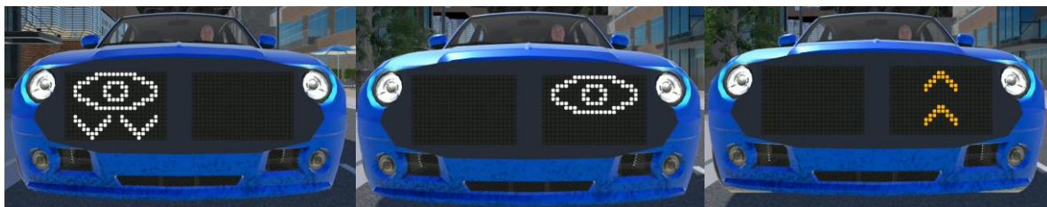
Figure 3-16: HMI 1 – Short-Term eHMI. (Left to right) message “slowing for pedestrian”, “stopped” and “accelerating / not stopping”.
