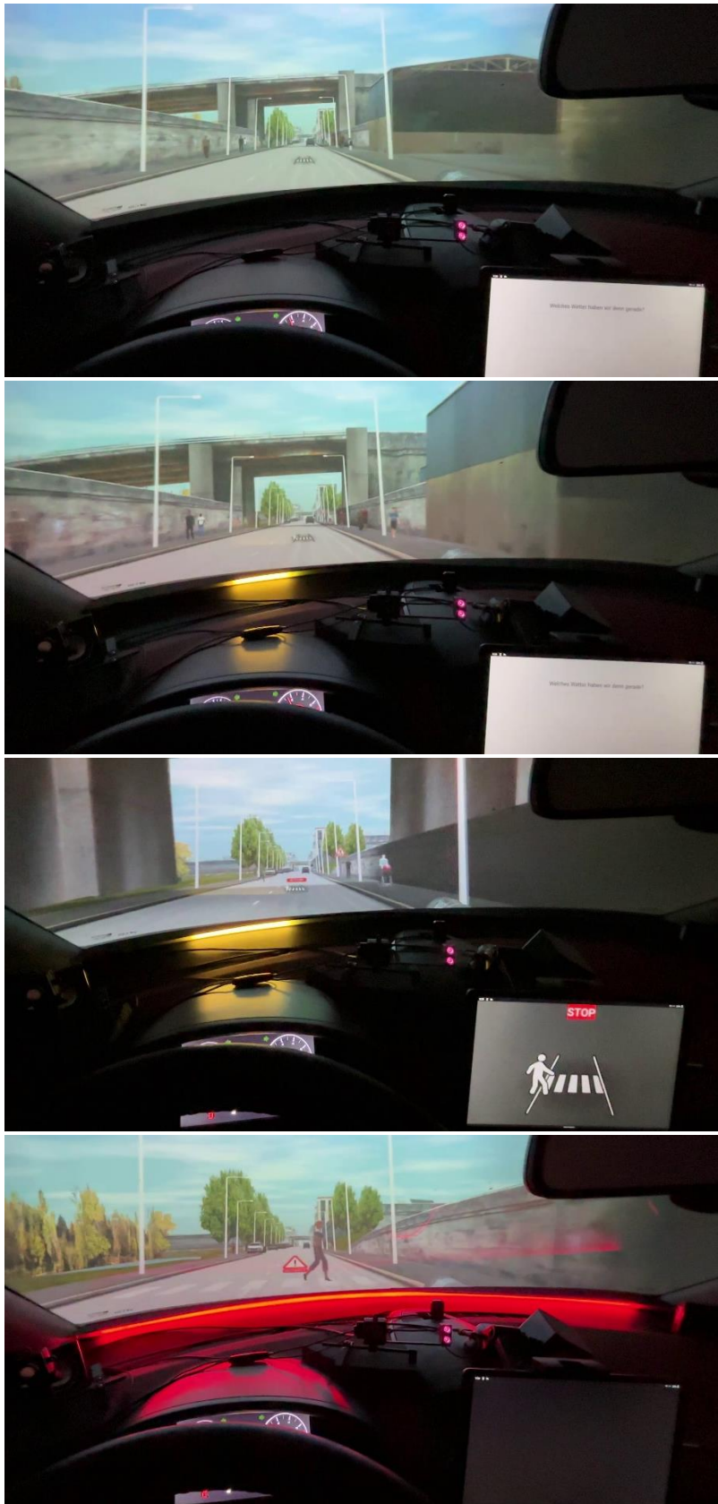
Figure 5-12: Different layouts of the regular iHMI when the driver is distracted.
