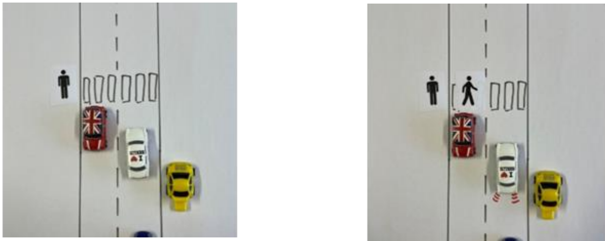
Figure 8-4: Situation 4: Pedestrian crossing from left side at zebra crossing hidden by oncoming vehicle
